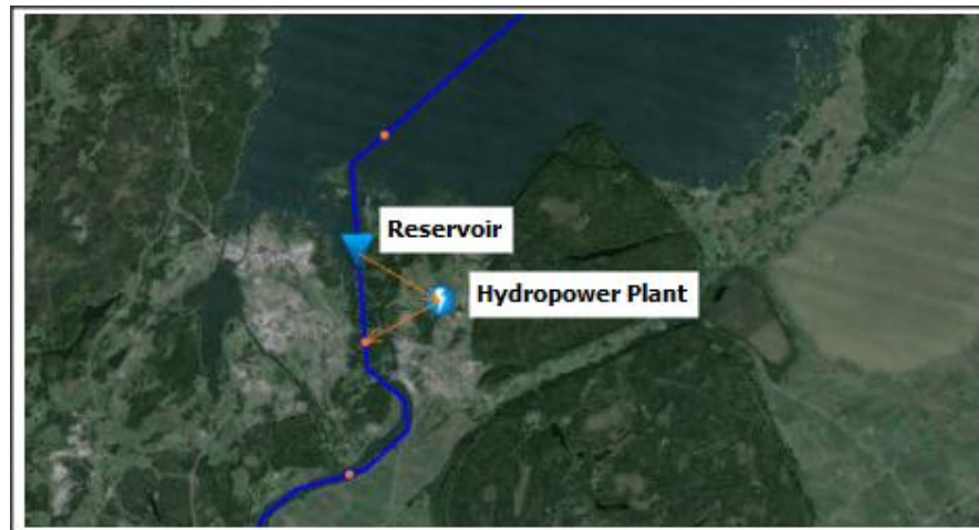
Figure 4: Hydropower plant defined with a single reservoir connection and return flow definition to river location downstream of reservoir
